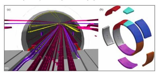
(a) Tunnel model including interior systems, (b) ring model including segments.
