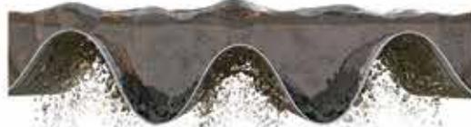
Gravity and vibration force the solids into the corrugated screen's troughs, thus allowing more fluid to pass through the top of the screen.
