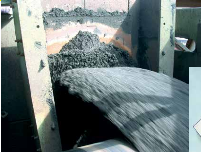
(left) KALIMPACT lining fitted to a bunker in a loading and unloading plant
