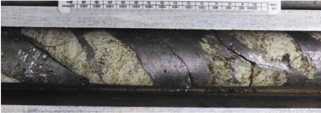
Sri Lankan vein graphite in granitoid host rock. Scale rule = 15 cm (~6 in.). Photograph: Andrew Scogings. Vein graphite sample by courtesy of Margosa Graphite Ltd.
