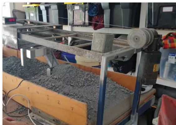
Fig. 1 Dozer test in action, showing winch, carriage, dozer blade and simulated muckpile.
