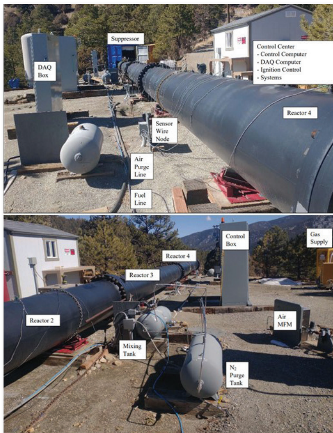
Fig. 1 Explosion reactor setup for large-scale experiments.
