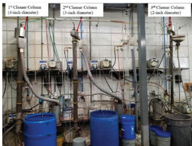
Fig. 2 Each zone of the three-stage cleaner column flotation.
