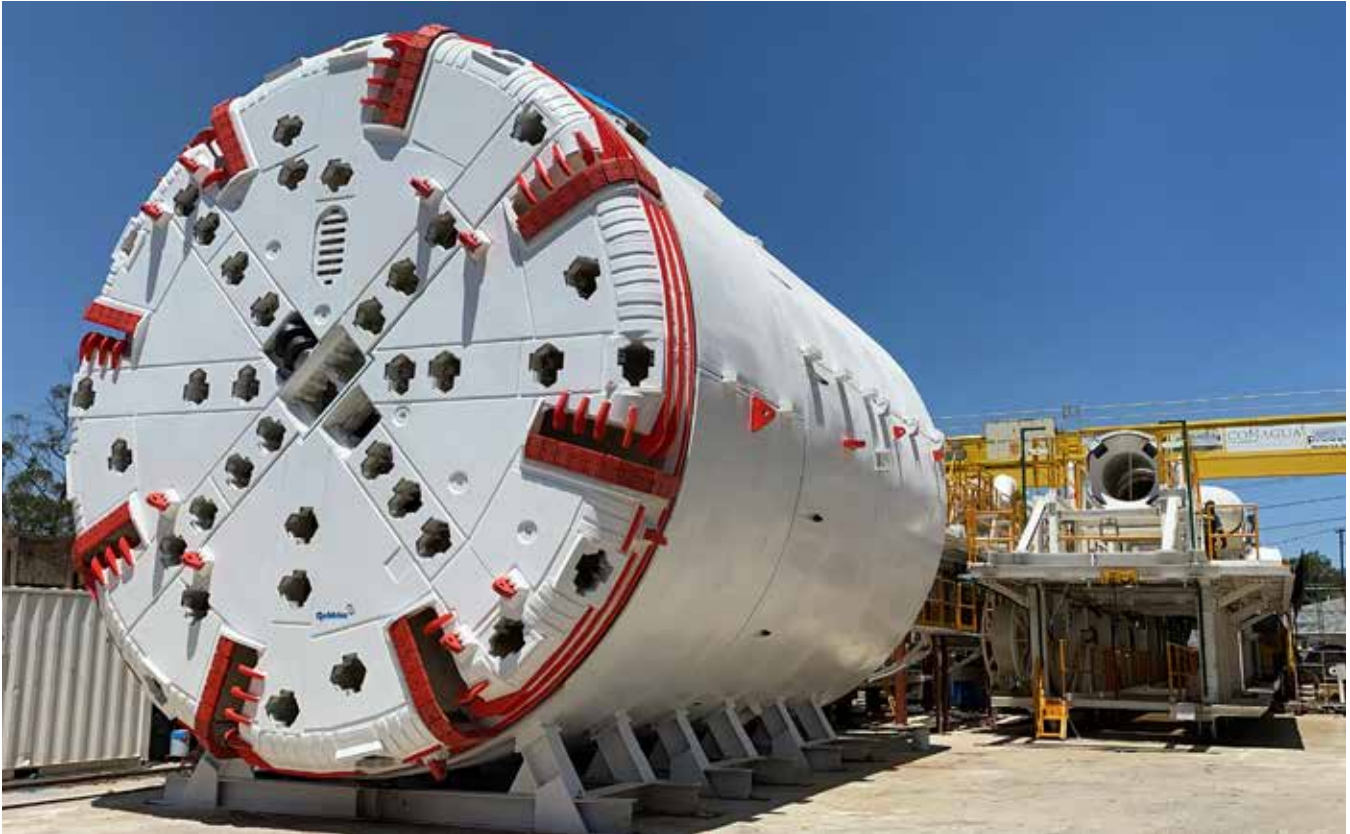
This Robbins TBM was originally built in 1995 and has been used on six tunnels around the world including in Laos, Mexico and most recently at Ashbridges Outfall in Canada.
