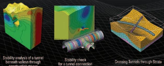
Stability analysis of a tunnel beneath valleys through construction stages      Stability check for a tunnel connection      Crossing Tunnels through Strata
