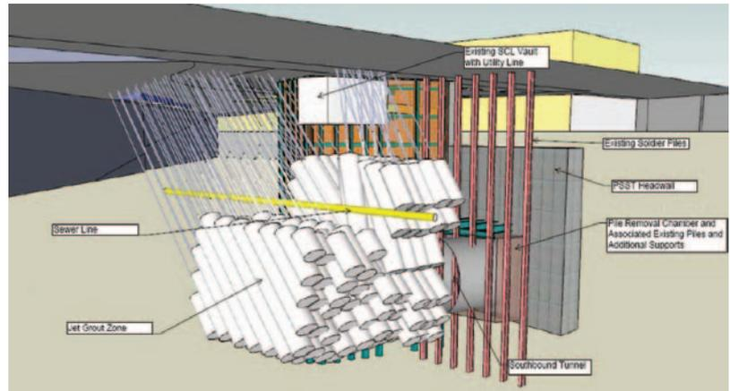
elevation 52 m (170 ft) to the base of the PSST structure. The layout of the piles avoids the electrical duct bank and the overhang of the existing vent structure.
