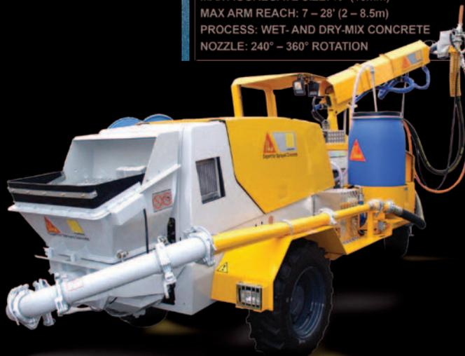
WITH ITS ALL-WHEEL DRIVE MOUNTING, TELESCOPING ARM AND SIGNIFICANT REACH CAPABILITIES, THE PM 407 ROBOTIC NOZZLE MANIPULATOR EASILY HANDLES A VARIETY OF SMALL AND LARGE UNDERGROUND APPLICATIONS SUCH AS MINES, TUNNELS AND PITS. ITS MODULAR DESIGN AND SIMPLE OPERATION PROVIDE MAXIMUM PARAMETER CONTROL, WHILE THE SWING-OUT HOPPER MAKES CLEANUP SIMPLE. FOR INCREASED PERFORMANCE, THE PM 407 IS AN UNDERGROUND OVERACHIEVER.
