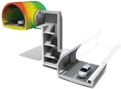
All types of T-type and Y-type interconnections, curved tunnels, shaft-lateral-main tunnel connections and tunnel entrances, as well as subway stations can be easily modeled in detail. A special feature exists for defining automated and realistic construction stages for sequential activation and deactivation of excavation segments, struc-
