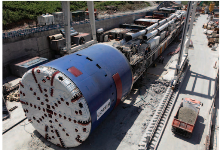
A Robbins Shield is excavating the 4.6-km (2.9-mile) main railway tunnel at Sochi, Russia's Complex #3.
