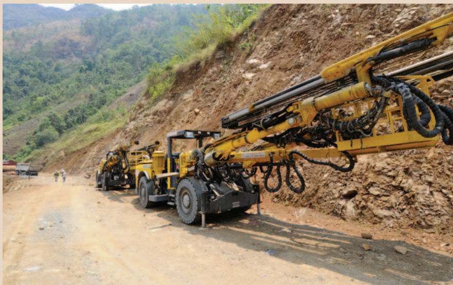
An Atlas Copco Boomer L2 D drill rig at work in Vietnam.
