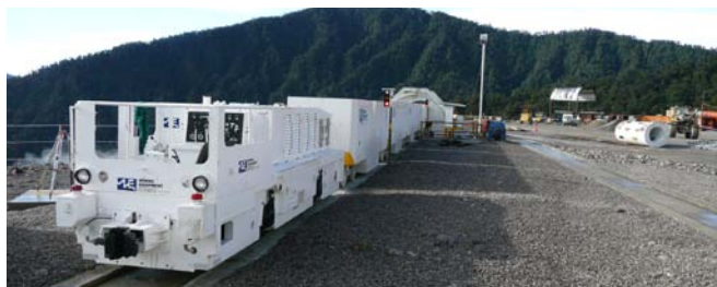
25-ton diesel locomotive pulling a string of 15 cubic meter capacity roll-over muck cars through a dump at their mine in Papua New Guinea.
