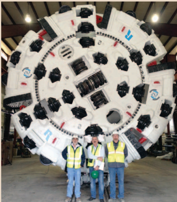
A Robbins main beam TBM is preparing to excavate the Indianapolis DRT for JV contractor Shea/Kiewit.
