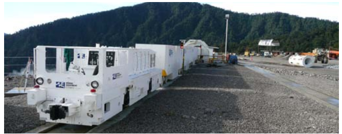
25-ton diesel locomotive pulling a string of 15 cubic meter capacity roll-over muck cars through a dump at their mine in Papua New Guinea.
