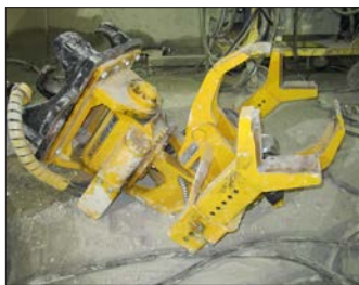
A close-up view of the beam manipulator designed specifically for the POMT project by Brokk's sister company, Kinshofer. Crews used the remote-controlled Brokk 400 and this beam manipulator to pick up and maneuver the steel support ribs into place in each cross passage.
