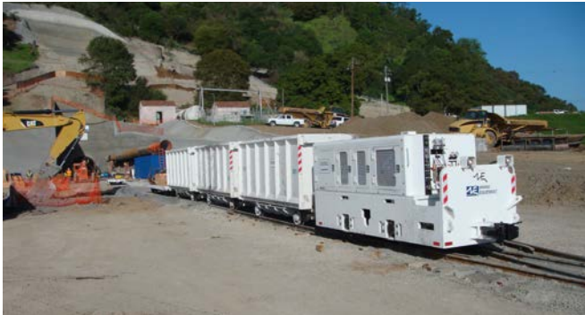
12-ton explosion proof diesel locomotive pulling 8 cubic meter side-dump muck cars out of the tunnel.
