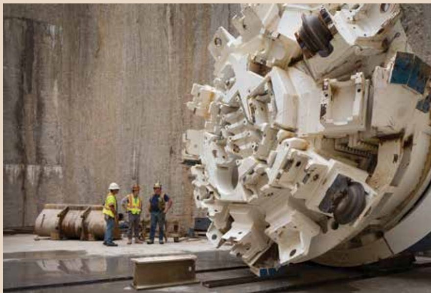
On April 30, 2015 in Honolulu, HI, a Robbins Main Beam TBM began a 4.6-km (2.8-mile) drive for a new sewer tunnel.
