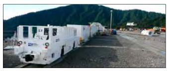
25-ton diesel locomotive pulling a string of 15 cubic meter capacity roll-over muck cars through a dump at their mine in Papua New Guinea.
