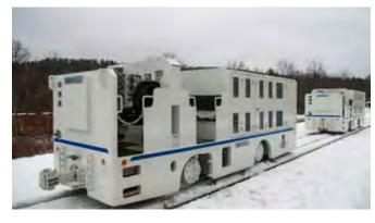
requirements. Featuring an 8.3L Cummins six-cylinder diesel engine and four-speed transmission, the 185-horsepower locomotives operate on 36-inch rail gauge underground for Walsh-Shea Corridor Constructors .
