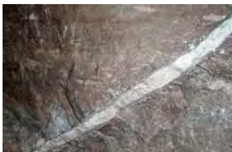
High mobility grouting of karstic rock enabled dry excavation of the OARS CSO shafts.
