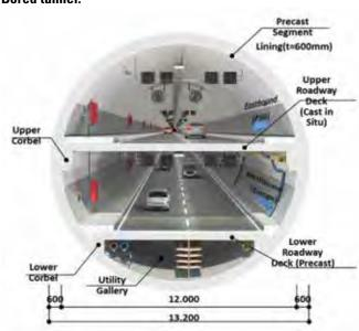
with precast concrete panels resting on similar corbels. The space beneath the lower deck accommodated the cableways, sump pumps, water and drainage systems, and other utilities supporting the tunnel operation.
