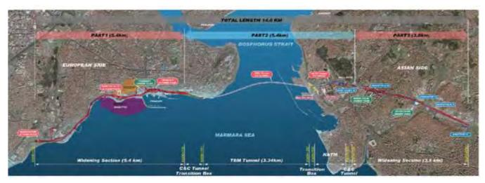
The 13.2 m (43 ft) external diameter, double deck Istanbul Strait Road Tube Crossing is one of the most challenging underwater tunnel projects in the world. Subjected to 11 bars of hydrostatic pressure, variable geology, and being in a very active seismic area, the execution of the project required innovative solutions, sophisticated construction techniques and
