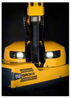
The Brokk 110 features hardened parts, LED headlight protection, reinforced corners and a new steel gray color coating in strategic areas to add additional resistance to dirt and scratches.
