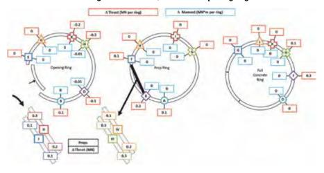
and accompanying slight relaxation in force. These effects are seen most prominently in the data for the prop ring and opening ring, which are partially exposed by the excavation.
