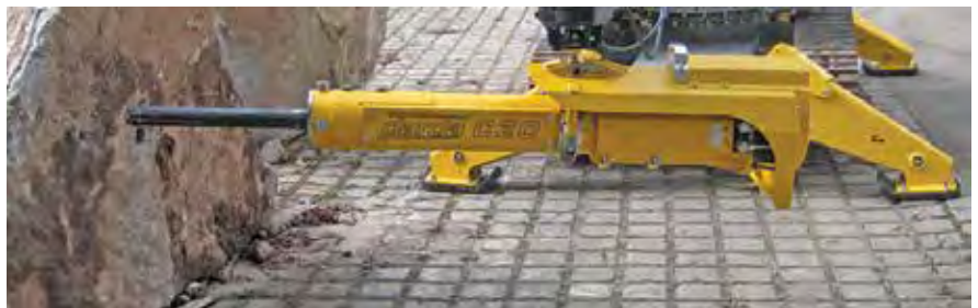
The C20 rock splitter can be quickly interchanged on a Brokk machine for greater versatility on a jobsite.
