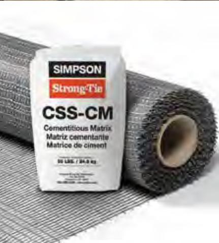
Repair, protect and strengthen aging, damaged or overloaded concrete and masonry structures in one application and significantly reduce your installed cost. The new **FRCM Externally Bonded Composite Strengthening System** combines high-performance sprayable mortar with carbon fiber mesh to create thin-walled, reinforced concrete shells without adding significant weight or mass to the structure.
