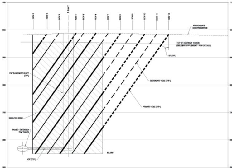
down and thickened and injection continued at the specified grout mix until changes in pressure or flow rate were observed. Typically, mix changes were made after 380-757 L (100-200 gal) of grout were injected or if it was immediately apparent that the interval was open and a thicker grout would be needed.
