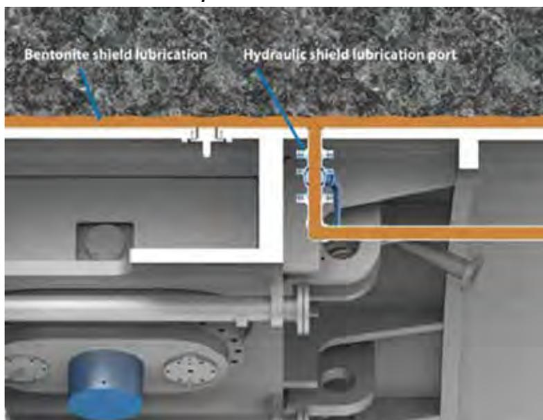
Field results have shown, time and again, that a TBM built with risk insurance-type features (such as probe drills, shield lubrication, etc.) can have a huge impact on a project's success in terms of schedule, cost and safety. It is better to build features into the machine from the start as part of a comprehensive risk management strategy, than to add them in the tunnel after an unforeseen event has occurred or the machine has become stuck.
