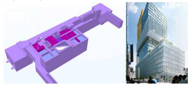
elements. Figure 5 illustrates the load transfer system in dark pink color to be built on the roof of the entrance structure for the future overbuild.
