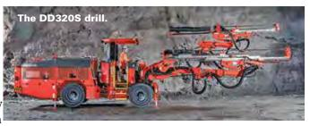
minimum downtime. It is optimized for 43-64 mm (1.7-2.5 in.) diameter bore holes and 76-127 mm (3-5 in.) reaming holes. Its carrier components, such as the diesel engine and layout, are similar to Sandvik DD321 technologies, ensuring common service principles and spare parts across the whole fleet.
