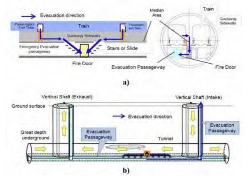
6a). The considered tunnel cross section provides sufficient space below the guideways to be used as an emergency evacuation chamber. The escape gallery would have an independent ventilation system in the event of a fire or other emergency and would have surface access via ventilation plants and shafts envisioned along the underground section of the alignment at an approximate distance of 5-6 km (3-4 miles) (Fig. 6b).
