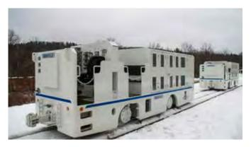
requirements. Featuring an 8.3L Cummins six-cylinder diesel engine and four-speed transmission, the 185-horsepower locomotives operate on 36-inch rail gauge underground for Walsh-Shea Corridor Constructors.
