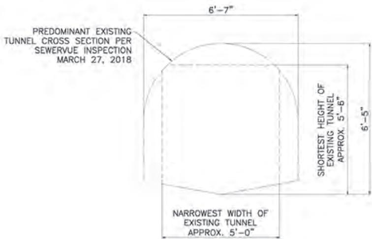
were carried out in 1981 and 1991 (Lachel & Associates 1991). In 2015, a multisensor robotic inspection was also performed (HDR Engineering 2016). This most recent condition assessment revealed that the tunnel needed rehabilitation and/or replacement due to deterioration of the shotcrete lining, ground water infiltration and other structural defects.
