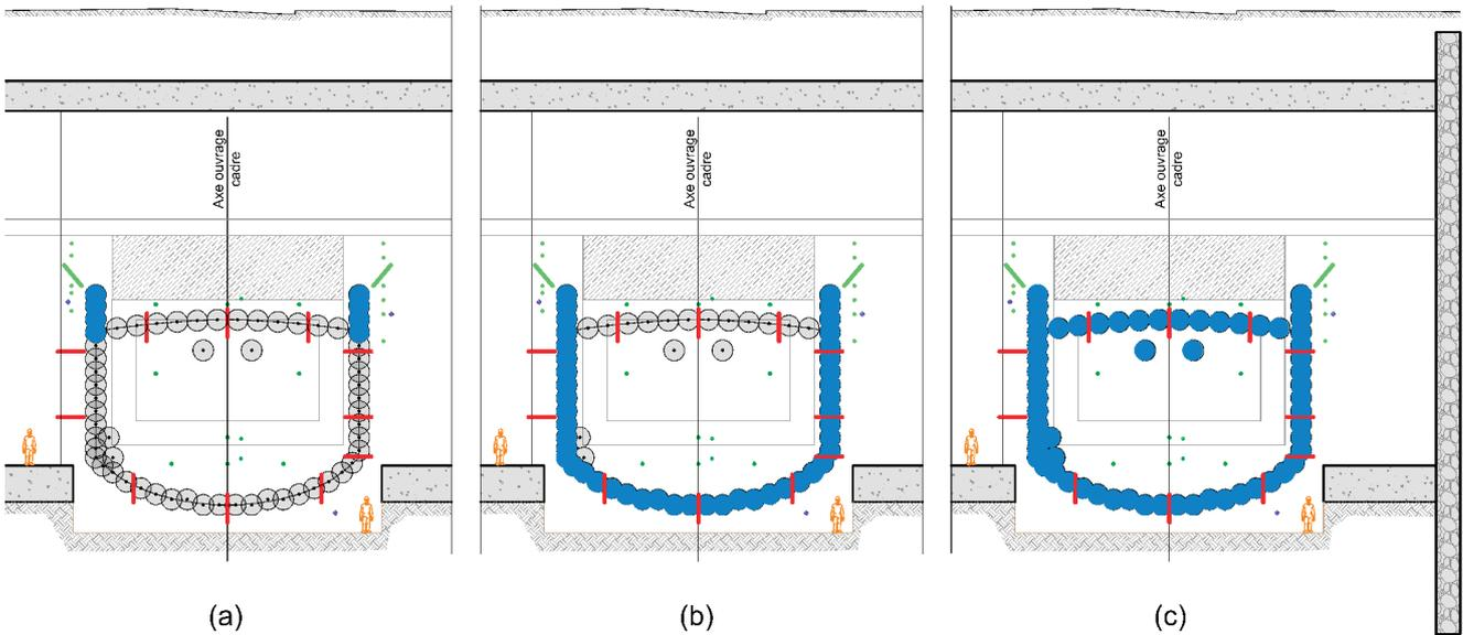
layer of fiber-reinforced shotcrete. Rib size was dictated by the rectangular shape of the galleries. Moreover, due to the geometrical constraints to drill the freeze pipes, the space between the frozen body and the excavation line was quite limited.
