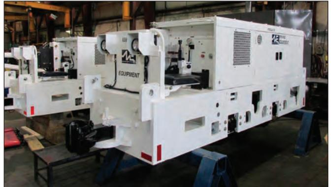
Mining Equipment 10 Ton Locomotives for Columbus, Ohio
