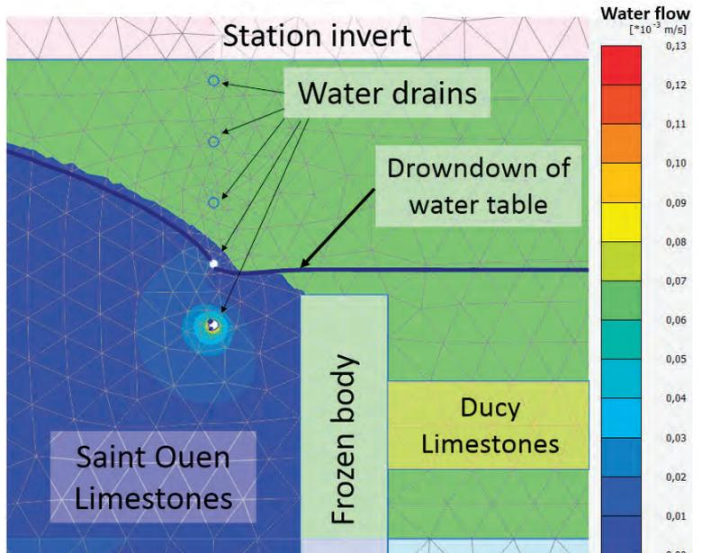
**Thermal erosion test.** Two drain lines were placed on either side of the gap between the upper freeze pipes and the bottom slab of RERC, to capture water seepage before it entered the tunnel. These drains were also used to reduce the volume of water that would flow over the U-shaped shell.
