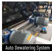
Auto Dewatering System
